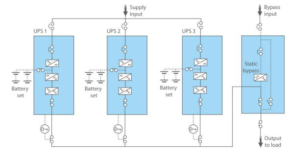
A typical N Capacity UPS System with Centralised Bypass Where each UPS is rated at 200kVA with the Centralised Bypass rated at 600kVA
