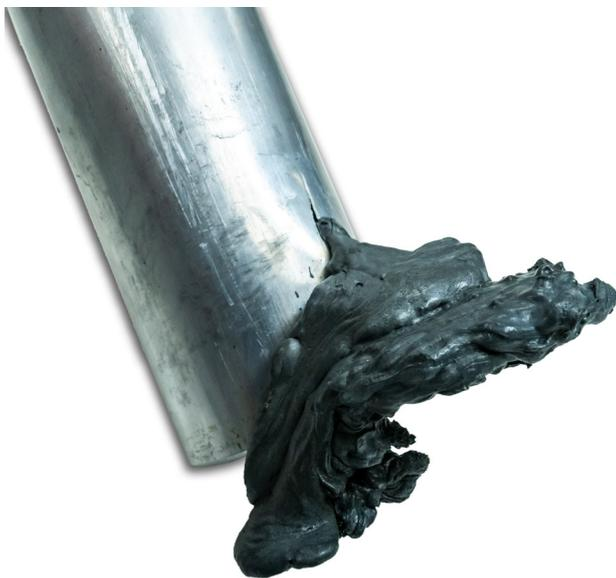
The electrolyte is conductive, so leakages can create unintended connections that could disrupt UPS performance. It is also corrosive, so is likely to damage any surrounding components.
